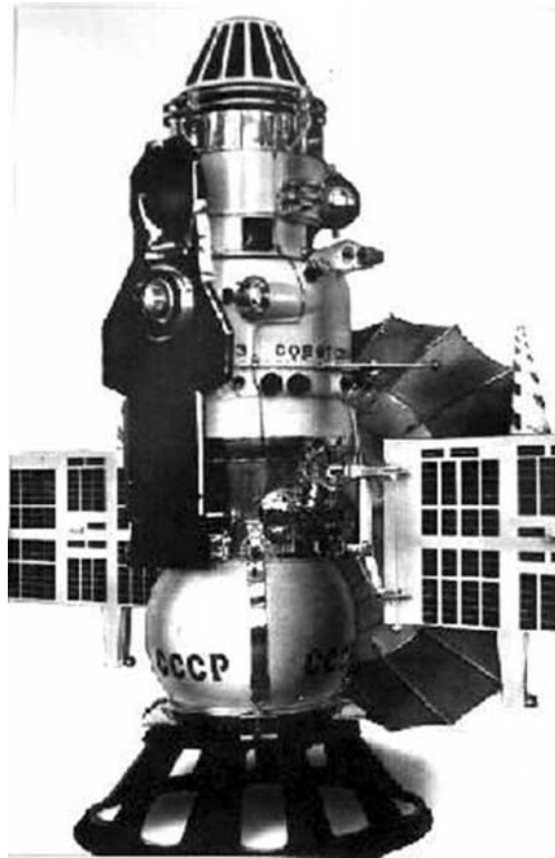
Figure 15. The Venera 7 spacecraft on a stand. Typical of the Venera 2–8 series, it consisted of a carrier vehicle with a propulsion module at one end (top) and a payload module, in this case a probe, attached at the other (bottom).
